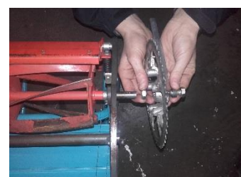
Figure 1: Assembly of driving gear to the mower
