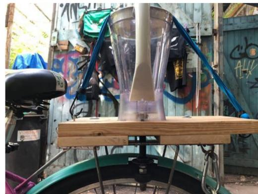
Figure 4. Completed smoothie stand and drive shaft
