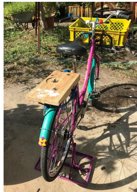
Bike in Smoothie Mode (With wing nuts on top of drive board)
