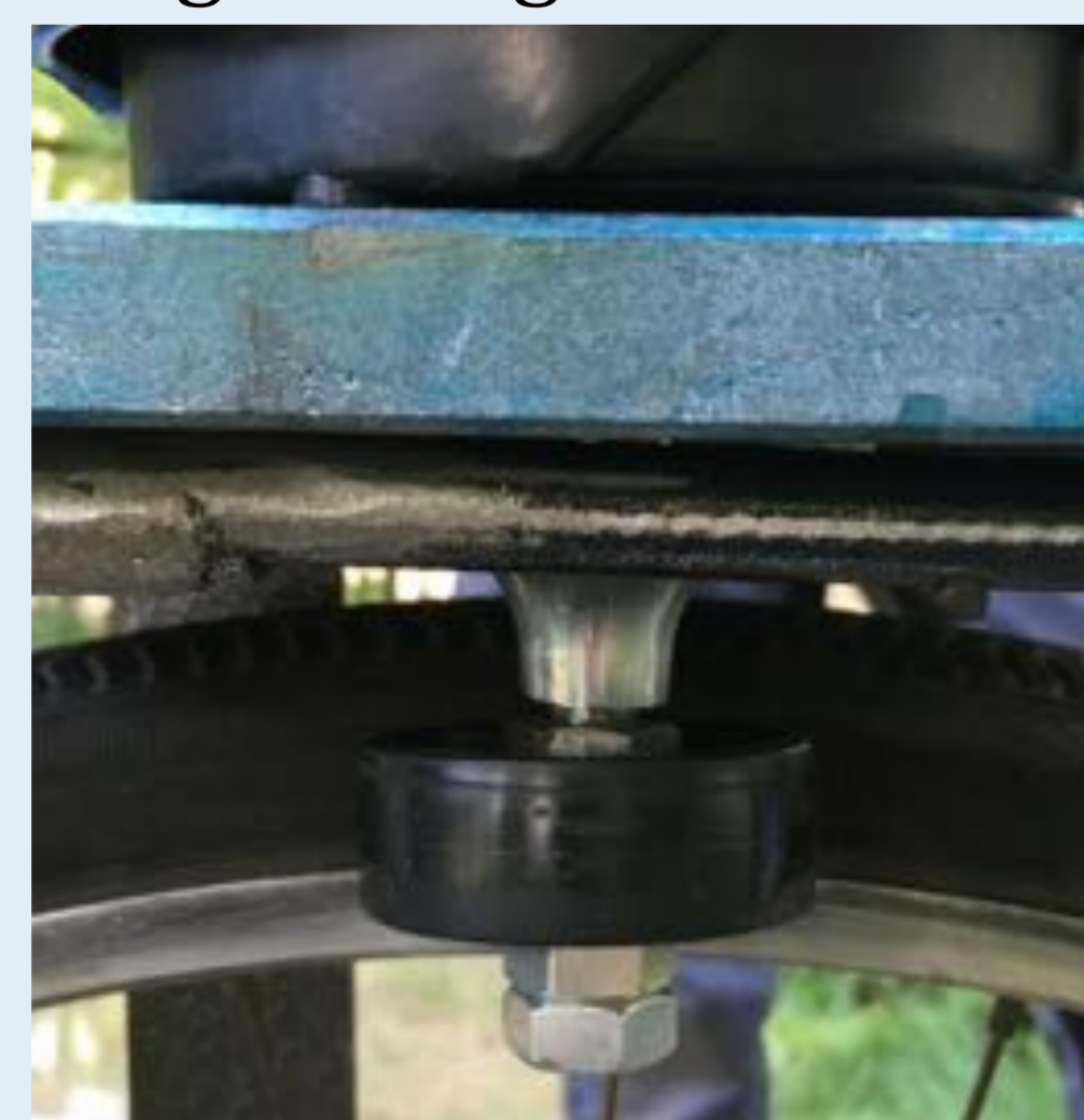
Friction drive contacting front wheel
