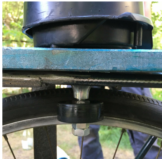
Blender drive assembled -- note proper contact with the bike tire for max efficiency
