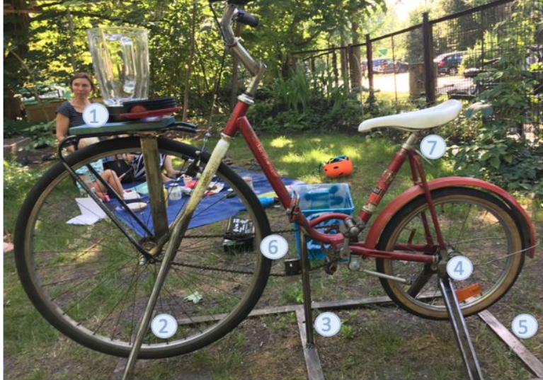
Bike components: 1) smoothie stand and blender, 2) front supports, 3) middle support, 4) rear supports, 5) support base, 6) chain tensioner, 7) adjustable seat.
